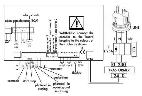
The current feed line (230V L,N, =) to the automation must be protected by a magnetometric switch or a pair of 5A fuses. A differential switch is recommended but not neccessary if it is already found at the top of the system.
